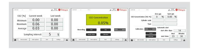
The internal data logger records each measurement and stores the values with time and date stamp and a user-defined name. The recordings can then be transferred via FTP to the computer.
