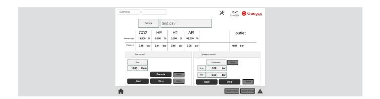
As an option, continuous gas analysis is possible, which ensures constant process and quality control. The integrated data logger enables complete documentation by recording all process parameters.
